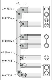
Fasteners with external and internal clamping technology for 90° connections can be used together. The effective profile length is identical. The 20 mm spacing must be factored in.
