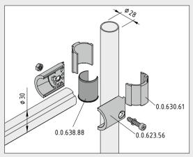
Thanks to Adapter D30/D28-37, it couldn't be easier to make the transition to a whole new dimension: Simply attach the Adapter to the tube ( $\varnothing$  28 mm), place a Tube Adapter D30 over it and the way is clear for extending your old structure using the innovative Profile Tube System D30.
