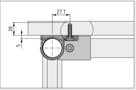
The clip of Table-Top Fastening Set D30 is laid over the Tube D30 and fastened directly to the table top with the enclosed screw, which is driven through the plastic spacer.
