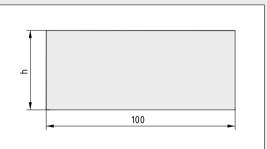
Recommended size of label cards: Label Holder D30: h = 28 mm Label Holder D30 flex: h = 42 mm
