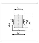
Roller Conveyor St D30 with Flanged Wheel
