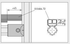
A section has to be cut away from the underside of the Cable Guide Profile so that it can fit perfectly over the contours of Fastener D30. This cutaway section must be at least 45 mm long and must be made at a height of between 14.3 and 19.5 mm.
