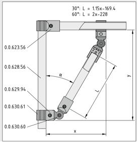
The length of connecting profile L is determined by the fastening elements that are used.
