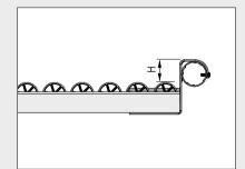
Roller Conveyor St, Fastening Brackets D30 with Stop are available with stops of different heights – H= 27 mm or 43 mm.
