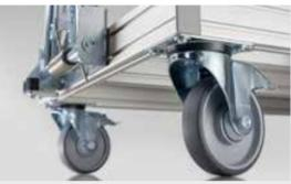
Swivel and Fixed Castors can be fixed to frames made using Line 8 profiles via the four holes in the integrated connecting plate. Alternatively, the Castors can be fixed to two parallel Profiles 8 D30. These tubes from Profile Tube System D30 feature an integral Line 8 groove. The corresponding Fastening Set 8 for Castor swivel/fixed makes installation easy.
