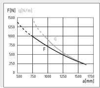
Permissible loads for constructions built with Tube D30.
