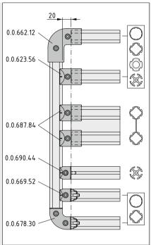
Fasteners with external and internal clamping technology for 90° connections can be used together. The effective profile length is identical. The 20 mm spacing must be factored in.
