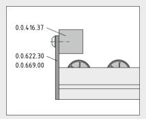
If required, you can terminate the Castor Rail by fitting an Impact Buffer (see Comprehensive Catalogue for MB Building Kit System) to the Cap.
