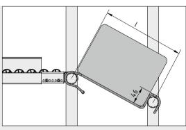
The length of the Slide Links has been matched to the dimensions of transport boxes. An additional section of tubing secures the top ends of the wire against lateral movement.
