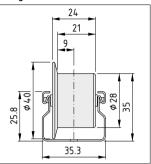
Roller Conveyor St D30 with Steel Tyres
