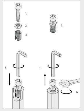
Threaded Inserts, Profile Tube D30 heavy duty can accommodate extraction forces of up to  $F_{\text{max}}=20000\ \text{N}$ . The load limits of Profile Tube D30 heavy duty and the screw (particularly in the case of an M6 diameter) must be factored in for constructions.
