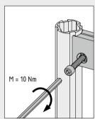
Profile Tubes D30 that are connected using Transverse Fastener D30 are spaced 18.5 mm apart. When using Tube Adapter D30 (0.0.630.61), this gap increases by 5.5 mm per side.
