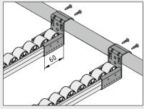
Roller Conveyor St Fastening Bracket D30 can be fixed in place in a matter of seconds with the self-tapping Button-Head Screw – simply use a cordless driver to drive the screw into the (Profile) Tube D30.
