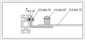
The pin of Drawbar Coupling D25-74 (0.0.661.87) should be pointing up when using Drawbar D25-686 (0.0.664.13). By contrast, when using Drawbar D25-686, Self-Lifting (0.0.664.12), the pin should be installed pointing down. The Coupling is fitted to the 80 mm-high Line 8 profile of the load-carrying frame using the groove indicated above and two Fastening Sets 8 6-8mm with Hexagon Socket Head Cap Screw M8 (0.0.684.91).
