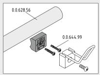
The adapter can also be fastened to Tube D30. Self-tapping screws (0.0.644.99) are used in this case. The retaining plates must be removed from the adapter.
