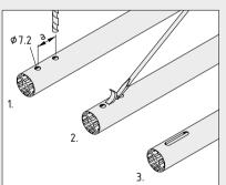
Any covered grooves on a profile can be opened up as and when required. The openedup section of the groove can be used in the usual way to fasten accessories or panel elements.
