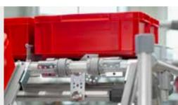
Rollers D46/D30-20 and Fastening Rings D40/D30-10 must be pushed onto the (Profile) Tube D30 before the tube is fitted into place.
