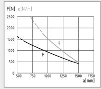
Permissible loads for constructions that use a combination of Profile Tube D30 and Bracing Strut D30-90°.
