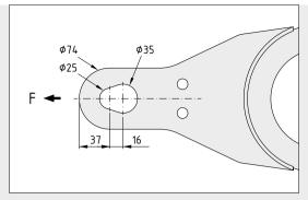
Rated tensile force in continuous operation = 6000 N Maximum rated trailer load in continuous operation = 6 t
