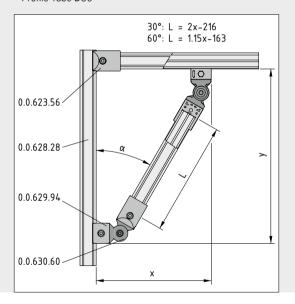
Tube D30 with Tube Adapter
