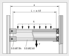
Calculating the necessary length of Double Profile Tube D30-60 when using Fastener D30 T1 and Fastener D30, internal.
