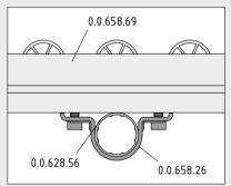
Brackets D30 can be used to secure crossmembers directly underneath roller conveyors with a Line 6 or 8 groove.
