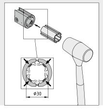
Another option for removing the anti-torsion features that does not involve dismantling the preassembled fastener halves is to break them off with a hammer and a section of profile.
