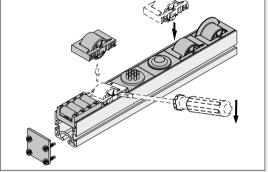
Customising Castor Rail 8 40x40 couldn't be easier: Simply push the inserts into the rail to build your ideal roller conveyor. Caps secure the ends.
