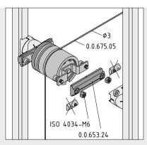
Adapter 8 80 D30 (0.0.653.24) can be used to attach Braking Roller Set D52-95 M6 to a Fastener D30, although the two anti-torsion features of the Adapter must be removed in order to do so.
