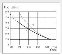
Permissible loads for constructions built with Tube D30.
