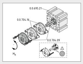
Bearing Block 8 80x80-50 (0.0.695.21) can be fitted with up to three rotational dampers, as required. Rotational Damper Set T1 (0.0.704.09) uses a square spindle as an axle. To prevent injuries, this spindle must be cut to size if fewer than three rotational dampers are being used on Bearing Block 8 80x80-50.
