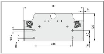
Fastening dimensions for Drawbar D25-686 and Drawbar D25-686, Self-Lifting
