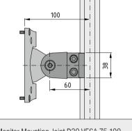
Monitor Mounting Joint D30 VESA 75-100 features two independent joints. As a result, it can be used to pivot the screen to the side and tip it to find the right viewing angle.
