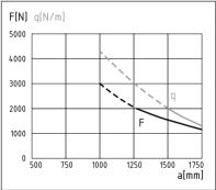
The diagram shows the permitted load in relation to support span a. It is based on the maximum permissible deflection set by item, which is 1/100 of the support span. When designing rack structures, please observe the limit values set out in the relevant statutory regulations (e.g. DGUV regulation 108-007 in Germany).
