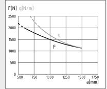
Permissible loads for constructions that use a combination of Profile Tube D30 and Parallel Fastener D30.
