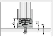
When using End Connector 8 D30-90° on a component with a smooth, unbroken surface, all four tabs of the integrated anti-torsion features on the connector adapter must be removed. An M6 nut can be inserted into the connection adapter to create a screw connection from the rear.
