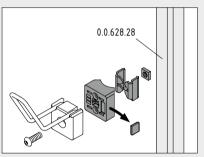
When connecting to vertical struts, the removable anti-torsion feature in the plastic block of the Hook and Holder Adapter must be removed.
