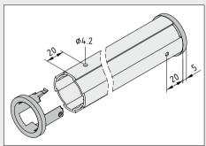
When building custom plain bearings in lengths of over 50 mm, four holes need to be drilled in the Profile Tube D40/D30 (0.0.666.63) to accommodate the tabs on the Plain Bearing Sleeves.
