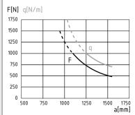
Permissible loads for constructions built with Profile Tube D30-45° heavy duty and Profile Tube D30 heavy duty.
