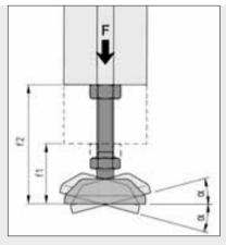
A ball and socket joint compensates for slopes.
