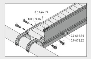
When Guide Rail e 4 reaches up to the supporting crossmember, the Roller Conveyor 60 Fastening Bracket D30 can be screwed into place on just one side.
