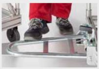
To couple and uncouple Drawbar D25-686, Self-Lifting, the operators use their foot to press down on the Drawbar, which is kinder on their back. A spring lifts the Drawbar up, ensuring that it is securely held against Drawbar Coupling D25-74, which features a downward-pointing pin.
