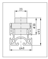
Roller Conveyor 8 D30 with Flanged Wheel
