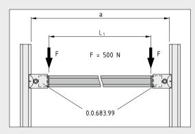
Profile length  $L_1$  varies depending on the profile and Threaded Insert used. Both bearing units of Pivot Bearing Set D30-28.5 M8 are fastened at the ends of the profile. Loading values F correspond to those of Profile Tube D30.
