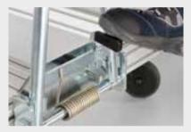
Drawbar Locking Lever 38 keeps coupling elements neat and safe. It holds the Drawbar securely in a vertical position, which is particularly advisable when using the version without a self-lifting mechanism. The foot-operated lever ensures the locking lever can be released without having to stoop down.
