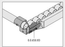
A Retaining Plate, Guide Rail e (0.0.650.83) can also be fitted to the side of Guide Rails e to provide additional support. They are screwed into place using self-tapping screws driven through the lower holes in the Retaining Plate.
