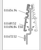
Guide Rail e 4 is screwed to Roller Conveyor St 60x24 D15 using Button-Head Screws self-tapping St 3.9x16 (0.0.642.39).
