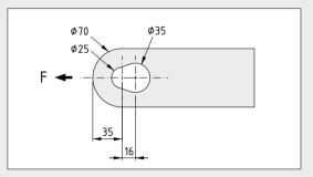
Rated tensile force in continuous operation = 3000 N Maximum rated trailer load in continuous operation = 3 t
