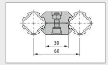
Parallel Fastener D30-60 and Parallel Fastener D30-60 with Clamp Lever connect Profile Tubes D30 and Profiles 6 D30 in the modular dimension. When using Tube Adapter D30 (0.0.630.61) and Adapter 8 D30 (0.0.630.51), the gap is larger.
