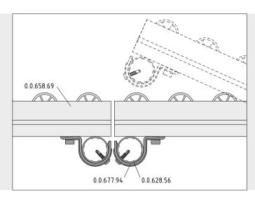
Compact Brackets D30 T2 are used when components pivot past each other or when there is little space due to the installation scenario. Bracket D30 T2 and the (profile) tube must be screwed together using the self-tapping screw supplied with the bracket.
