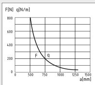
Permissible loads for constructions built with Tube KH D30x11.6.
