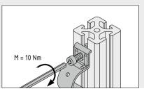
When screwing Brackets D30 to profiles, a tightening torque of 10 Nm should be used. By contrast, the maximum tightening torque when fitting the brackets to aluminium roller conveyors (Roller Conveyors 6 40x40 and 80x40 and Roller Conveyor 8 D30) is 5 Nm.
