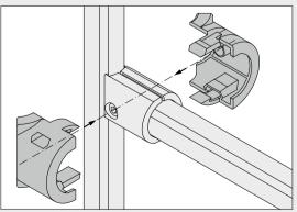
Protective Cover R28 for Fastener D30 comprises two half shells that can be removed without leaving a trace. To loosen a Fastener that is encased in a Protective Cover, simply push through the point marked with a dot.
