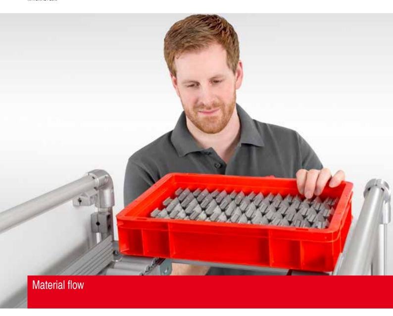
Getting your production in full swing: Roller conveyors are an efficient solution for organising material flow. Containers, finished parts and consumables roll almost effortlessly to the station where they are to be used. item roller conveyors can be suspended on frames or boost the stability of a mobile transport solution as a load-bearing element.
