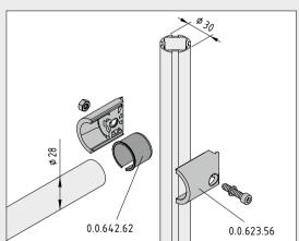
Connect a steel tube (Ø 28 mm) to an item Profile Tube D30 simply by inserting Adapter D30/D28-25 into an item Fastener D30 and the connection will hold firm.
