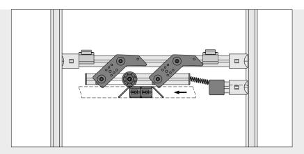
A Release Unit D30 Actuator Roller operates at least two Bars at once and can operate more, if necessary. Depending on the width of the load, a second roller conveyor can be secured simply by adding an additional Bar.
