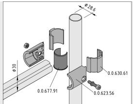
Depending on the connection type, a steel tube ( $\varnothing$  28.6 mm) can be connected to an item (Profile) Tube D30 using either the shorter Adapter D30/D28.6-25 (0.0.677.92) and a Fastener D30 (0.0.623.56) or the longer Adapter D30/D28.6-37 (0.0.677.91) and a Tube Adapter D30 (0.0.630.61).
