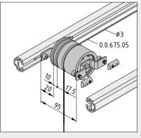
Braking Roller Set D52-95 M6 comes with four T-Slot Nuts and matching screws so it can be installed between two Profile Tubes 8 D30 or other profiles with a Line 8 groove.
