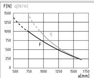
Permissible loads for constructions built with Profile 6 D30.
