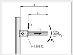
Double Pivot Bearing Unit D30-28.5 M8 can be fitted to just one end of a profile, via the end face. The required profile length  $L_2$  is determined by the combination of Threaded Insert and profile. In addition to the maximum load-carrying capacity of the Double Pivot Bearing Unit, it is important to also take into account the load limits of the adjacent components.
