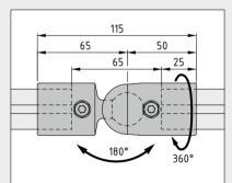
More freedom for your ideas! Ball Joint Transverse Fastener D30 allows you to position Profile Tubes D30 at any angle to each other. It provides a stable connection between crossing struts, such as those used to reinforce a frame. Crossing connections like these can be retrofitted extremely easily.
