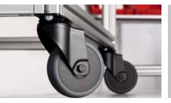
Perfect for small, manoeuvrable trolleys: item Castors D100 swivel are supplied with an integrated, narrow connecting plate. This means the swivel castors can be secured in place without the need for additional base plates. Featuring two holes, the connecting plate can be screwed to the profile grooves or the core bore of Line 8 profiles.
