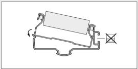
Roller Conveyor St 60x24 D15 is pressed into Fastening Profile D30-60 using a little force or can be slotted into place during assembly.
