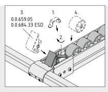
First, remove 2 roller elements. Insert the retaining plate in the direction of travel (1.) then twist into place (2.). Next, insert the Back Stop (3) for Roller Conveyor 6 40x40 E D30 and one of the two roller elements you removed earlier (4.).
