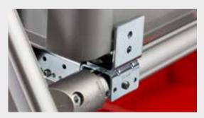
As Roller Conveyor St Stop H43 is not mounted to a crossmember, users can build roller conveyors that project outside a frame and thus reduce reaching distances. Light transport boxes are brought safely to a halt. The stop must be screwed to the Roller Conveyor St D30.
